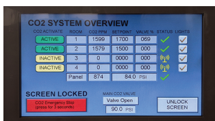
A closer look at enVgrow's display showing all zones monitored. The system will display warnings and notify you of any irregularities.
